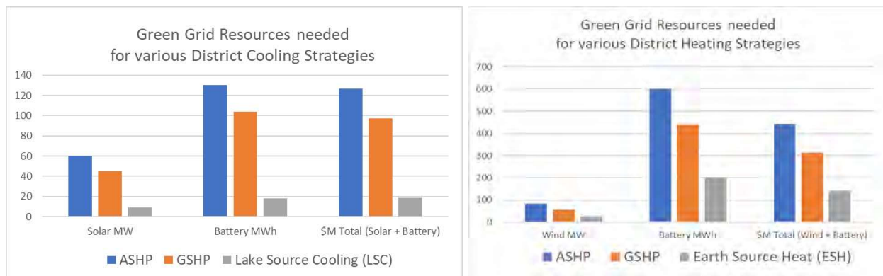
Figures 1a and 2b: Grid Resources for various district thermal strategies. Innovative renewable cooling (left) and heating (right) systems dramatically reduce the size of solar and wind farms, respectively, and battery storage systems needed to create a 100% renewable electrical grid compared to conventional Air Source Heat Pump (ASHP) and Ground Source Heat Pump (GSHP) technologies. Cost data is based on referenced National Renewable Energy Laboratory (NREL) reports.
